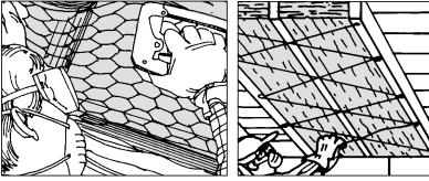
the joist cavity, staple chicken wire to the bottom of the joists OR lace wire back and forth around nails in the bottom of the joists.
