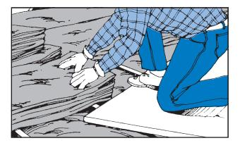
If you're adding a second layer of insulation, use unfaced insulation. Lay it across the joists. Work from eaves toward center of attic, butting insulation against wall at both ends.
