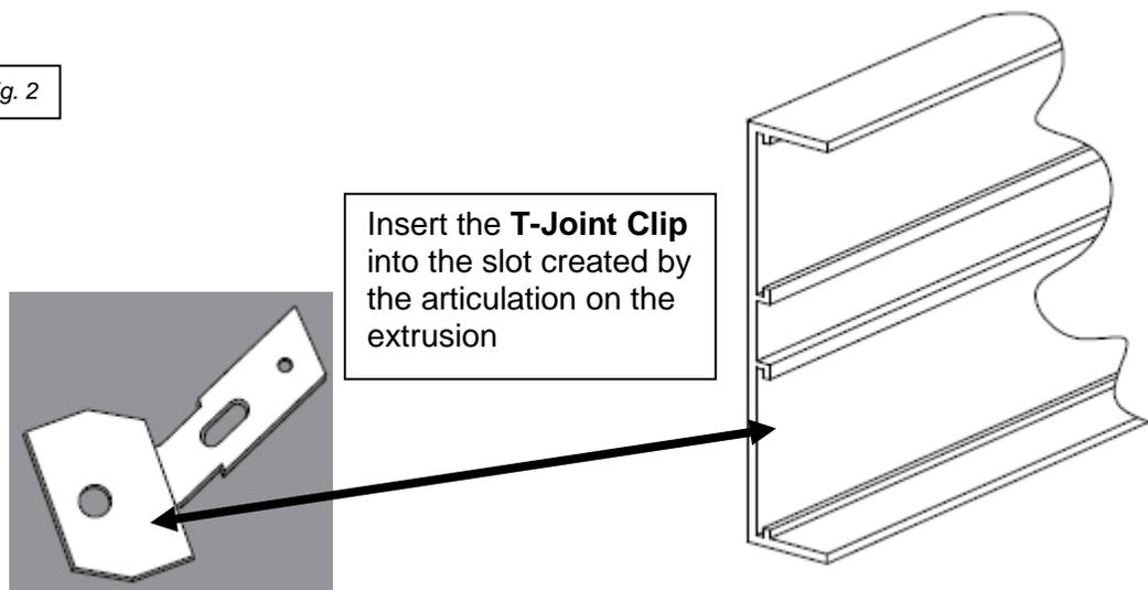
4. Attach the T-Joint Clip by means of a screw or rivet into the web of the cross-tee or main runner.
