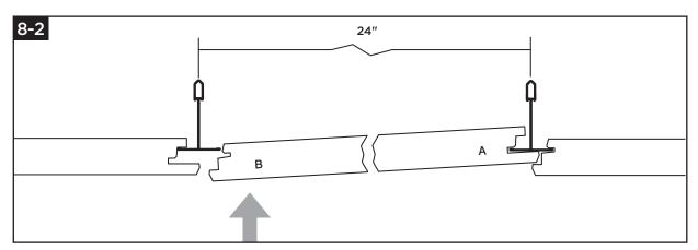
**Step 2:** While keeping light pressure toward edge (A), push edge (B) up to begin to engage the flange on the grid.
