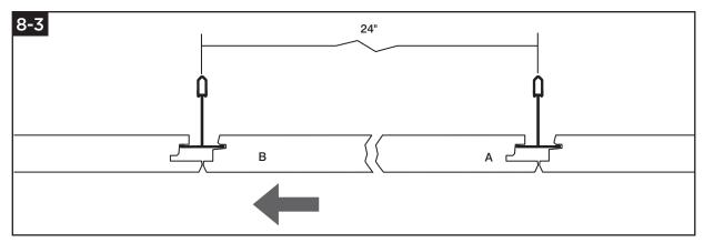
**Step 3:** Slide panel toward edge (B). Edge (A) will move into its finished resting place. To remove the panel, lift up gently on edge (A) and perform the process in reverse.
