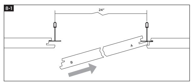
**Step 1:** Place the leading edge (A) into the grid as shown, making sure that the wider (deeper) groove is pushed as far as it can go into the flange. (This will allow the room to ensure that the trail edge (B) clears the grid on the opposing side).
