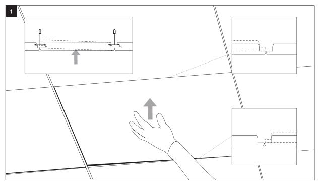
Place your hand on the center of the panel and gently push up to disengage the panel. Note: One edge will disengage higher than the other 3 sides.
