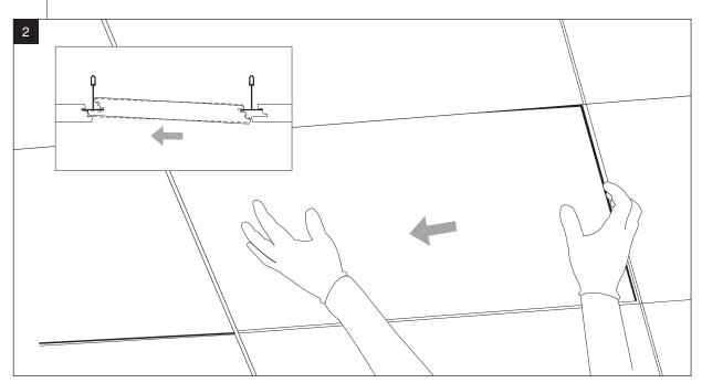
While keeping upward pressure, gently slide the panel toward the edge that has disengaged.
