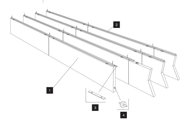
Ecophon Solo Baffle Anchor 1200mm x 600mm (≈ 47 1/4" x 23 5/8") 1200mm x 300mm (≈ 47 1/4" x 11 13/16") 1200mm x 200mm (≈ 47 1/4" x 7 7/8")
