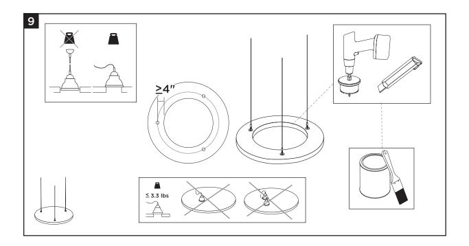
Installation for Ecophon® Solo™ Circle 800 Ceiling Panels — Connect Absorber Bracket Application
