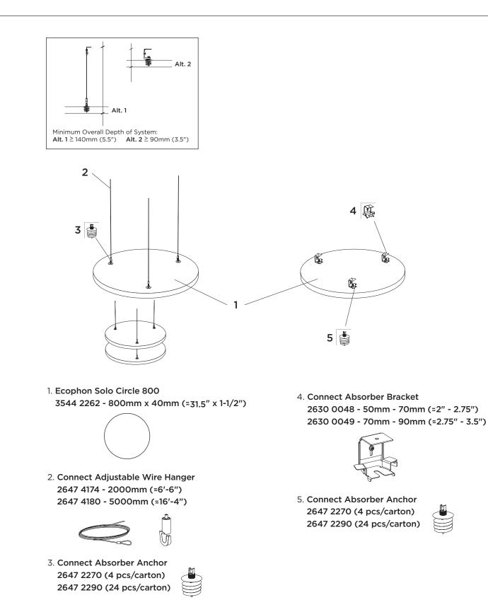
Installation for Ecophon<sup>®</sup> Solo<sup>™</sup> Circle 800 Ceiling Panels 800mm x 40mm (≈31.5" x 1.5")
