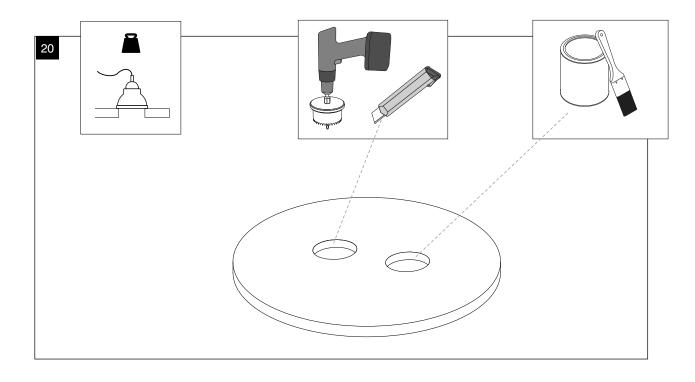
Installation for Ecophon® Solo™ Circle 1200 Ceiling Panels– Hole Placement With Panel Support
