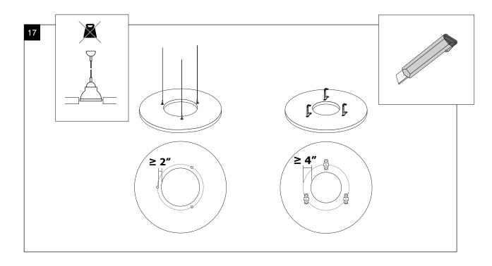
Installation for Ecophon® Solo™ Circle 1200 Ceiling Panels– Hole Placement Without Panel Support
