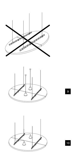
Installation for Ecophon® Solo™ Circle 1600 XL Ceiling Panels– Connect Adjustable Wire Hanger Application
