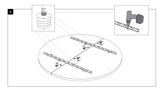
Installation for Ecophon® Solo™ Circle 1600 XL Ceiling Panels– Connect Adjustable Wire Hanger Application
