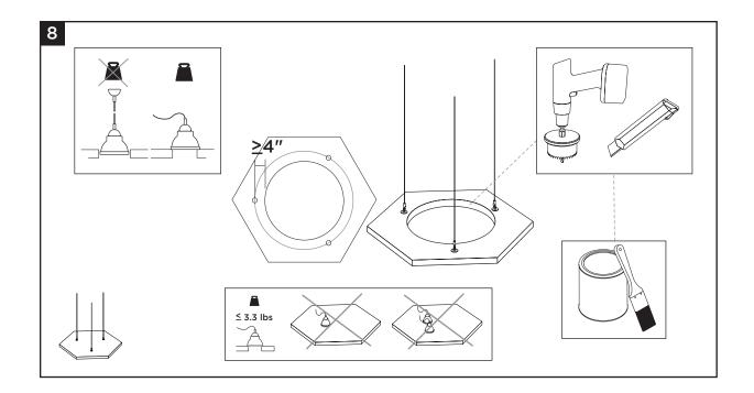
Installation for Ecophon<sup>®</sup> Solo<sup>™</sup> Hexagon Ceiling Panels — Connect Adjustable Wire Hanger Application
