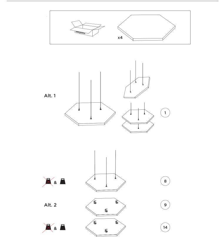
Installation for Ecophon<sup>®</sup> Solo<sup>™</sup> Hexagon Ceiling Panels — Connect Adjustable Wire Hanger Application
