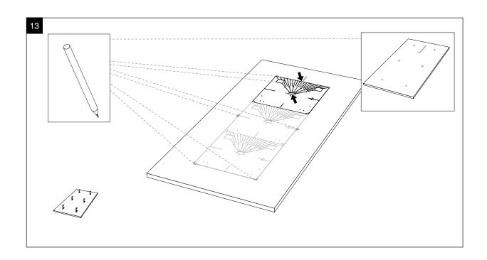
Installation for Ecophon® Solo™ Rectangle Ceiling Panel – Connect Adjustable Bracket Application
