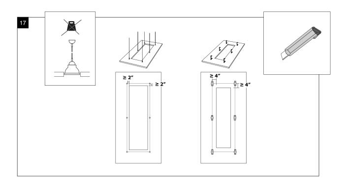
Installation for Ecophon® Solo™ Rectangle Ceiling Panel – Hole Placement Without Panel Support
