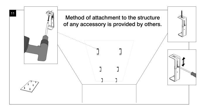
Installation for Ecophon® Solo™ Rectangle Ceiling Panel – Connect Adjustable Bracket Application
