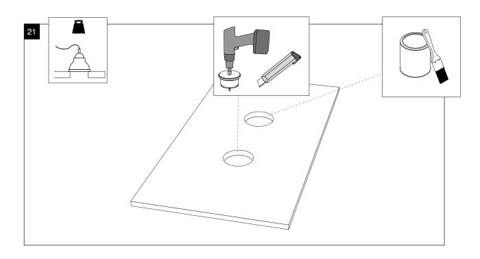
Installation for Ecophon® Solo™ Rectangle Ceiling Panel – Hole Placement With Panel Support
