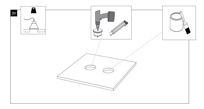
Installation for Ecophon® Solo™ Square Ceiling Panels– Hole Placement With Panel Support
