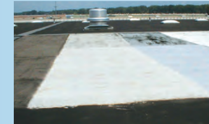
FlintCoat-W and FlintCoat-A after five years in service, with and without FlintCoat-E.
