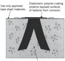
Fastener anchors itself in its own hole by cutting an inverted wedge of concrete. No pre-drilling required.
