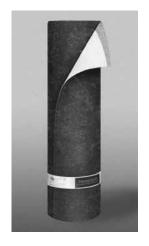
**Product Use:** Flintglas® MS Cap Sheet CoolStar® is designed for use as a cap sheet for hot asphalt applied built-up roof systems. It is surfaced with highly reflective CoolStar granules to provide a durable, heat-reflective weathering surface. It is suitable for both new construction and reroofing applications over a variety of substrates.
