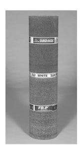
**Product Use:** Flintlastic® FR-P is designed for use as a cap membrane in SBS modified bitumen roof system assemblies over various types of substrates for both new construction and reroofing installations. It is suitable for most low slope roofing applications and may be used for roof system flashings including wall treatments, base flashings and field flashings.
