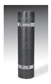
**Product Use:** Flintlastic GTA is designed for use as a cap membrane over various types of substrates for both new construction and reroofing installations. It is suitable for most low sloped roof decks and may be used for roof system flashings including wall treatments, base flashings and field flashings.
