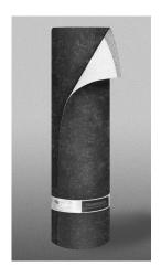
**Product Use:** Flintlastic® GTS-FR CoolStar® is designed for use as a cap membrane over various types of substrates for both new construction and reroofing installations. It is suitable for most low slope roofing applications and may be used for roof system flashings including wall treatments, base flashings and field flashings.
