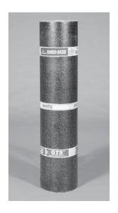
**Product Use:** FLINTLASTIC GTS is designed for use as a roofing membrane over various types of substrates for both new construction and reroofing installations. It is suitable for most low slope roofing applications and may be used for roof system flashings including wall treatments, base flashings and field flashings.
