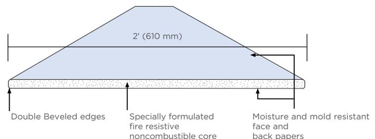
GlasRoc® and M2Tech® Shaftliner are designed and engineered for use in construction of lightweight Shaftwall and Area Separation Firewalls. These systems are UL, cUL, and ULC listed for fire resistance. GlasRoc® and M2Tech® Shaftliner can be substituted with each other.
