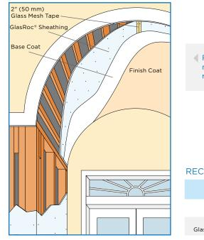
Refer to finish system manufacturer for glass mesh reinforcement requirements.
