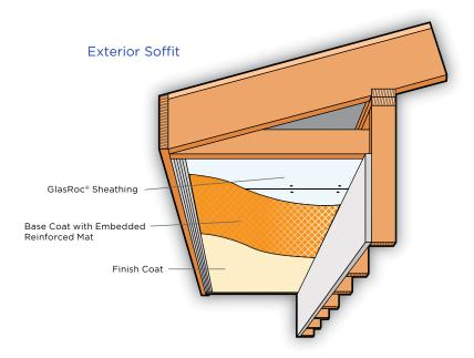
GlasRoc® Sheathing is a superior product for a flat ceiling entryway, exterior ceiling or a soffit assembly, due to its ability to resist the deteriorating effects of moisture and humidity.
