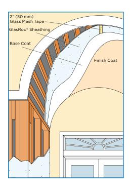
Refer to finish system manufacturer for glass mesh reinforcement requirements.
