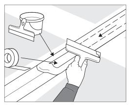
All board joints are to be filled with adequate joint compound. First, apply a layer of CertainTeed All-Purpose Joint Compound (or equivalent) in the tapered section. Next, add Marco Spark-Perf Paper Tape (or equivalent) in the wet compound. Lightly sand (100-200 grit) when cured. Apply a layer of CertainTeed All-Purpose Joint Compound (or equivalent). When cured, lightly sand until level with board.
