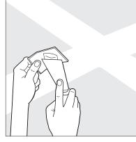
Fill screw heads with CertainTeed All-Purpose Joint Compound (or equivalent) in two rounds finished by light sanding until level. Tip: Use a piece of plastic with a circular hole as a mold.
