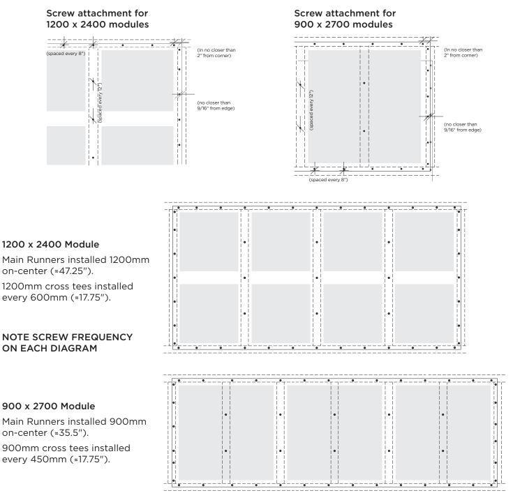
Installation of metal framing (CTA Drywall Grid System / metric) and Gyptone<sup>\*</sup> BIG<sup>m</sup> Boards
