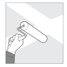
Paint Gyptone BIG with a 1/4" nap roller to avoid excessive paint into perforations. **DO NOT SPRAY PAINT BIG BOARD.** Gyptone BIG Boards is typically prime-painted once and finish-painted twice. Installation of metal framing (CTA Drywall Grid System / metric) and Gyptone<sup>\*</sup> BIG<sup>™</sup> Boards
