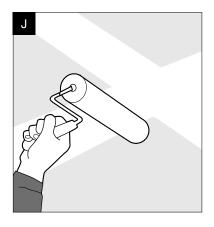
Paint Gyptone BIG with a 1/4" nap roller to avoid excessive paint into perforations. **DO NOT SPRAY PAINT BIG BOARD.** Gyptone BIG Board is typically prime-painted once and finish-painted twice.
