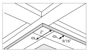
Install Gyptone BIG by using appropriate lifting equipment and fix to CertainTeed Drywall Grid with appropriate drywall screws. Use Gyptone QSTR 25 screws whenever fixing is necessary within the confines of any Gyptone BIG Boards perforated area.
