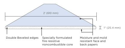
GlasRoc and M2Tech Shaftliner are designed and engineered for use in construction of lightweight shaftwall and fire walls. These assemblies are UL, cUL, and ULC listed for fire resistance. GlasRoc and M2Tech Shaftliner can be substituted with each other.
