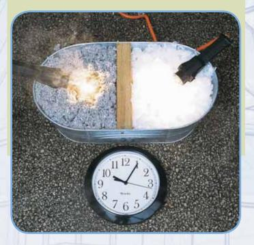
**After 15 minutes:** The light was removed from the cellulose, but combustion continued. There was no effect the on InsulSafe.
