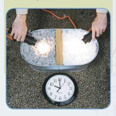
**After 30 minutes:** Combustion continued to spread in the cellulose. The light, inserted back into the InsulSafe, still had no effect.
