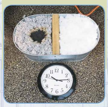
**After 47 minutes:** The combustion of the cellulose spread to the wood divider. There was still no effect on the InsulSafe.
