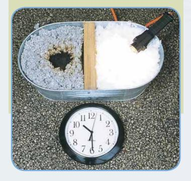
**After 5 minutes:** Smoldering combustion had begun in the cellulose side. There was no effect on the InsulSafe.
