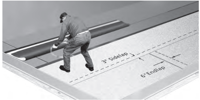
Figure 5-22: Remove the selvage edge release strip.
