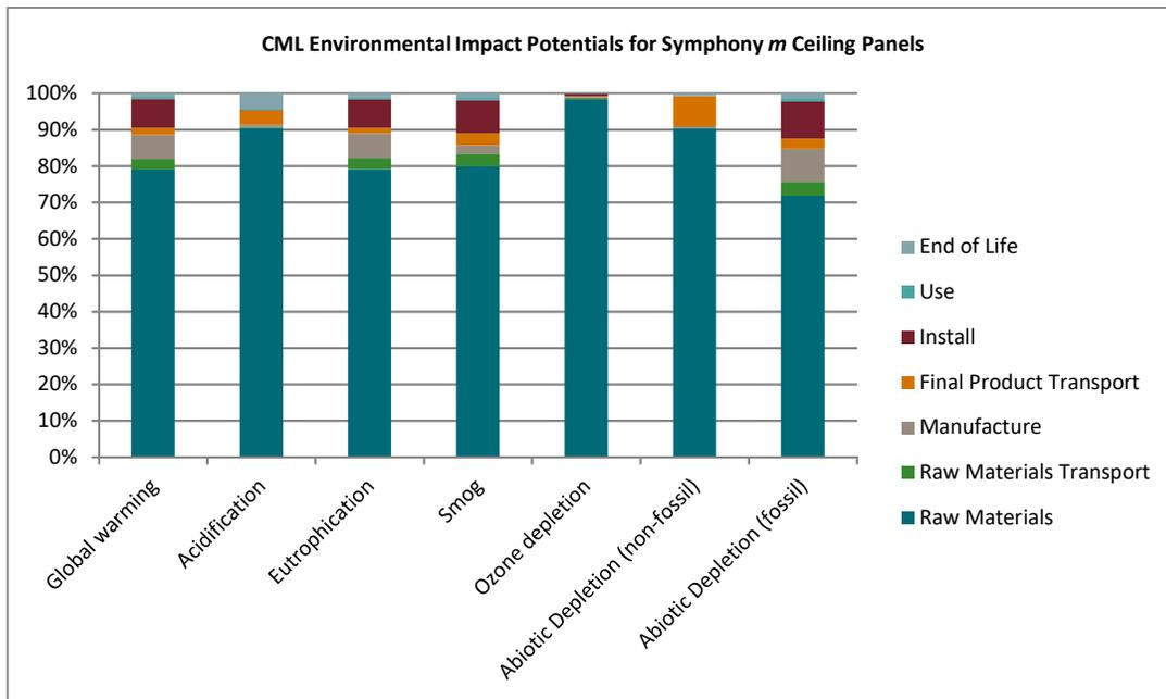
Figure 5: CML Environmental Impact Potentials for Symphony *m* Ceiling Panels per ft<sup>2</sup> (Outside North America)
