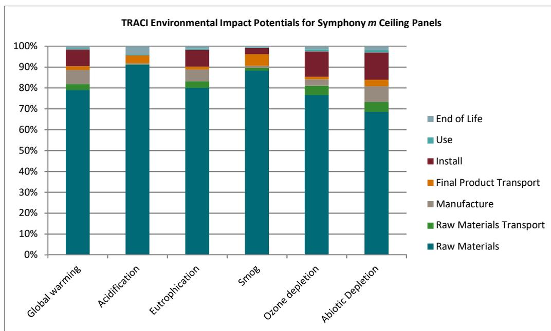
Figure 4: TRACI Environmental Impact Potentials for Symphony *m* Ceiling Panels per ft<sup>2</sup> (North America)
