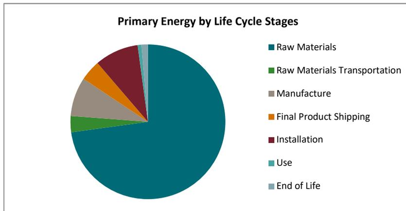
Figure 7: Symphony m Ceiling Panel Primary Energy by Life Cycle Stage
