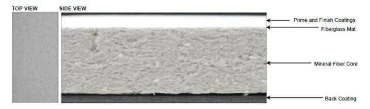
Figure 2: Diagram of Symphony m Ceiling Panel Construction
