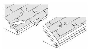
Figure 10-14: Preparing an old roof for reroofing.
