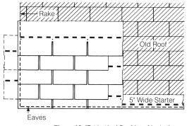
Figure 10-17: Vertical Racking, Nested.
