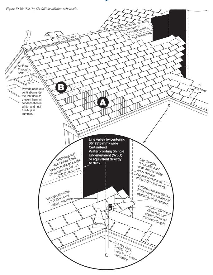
Figure 10-11: Highlight of closed-cut valley details.
