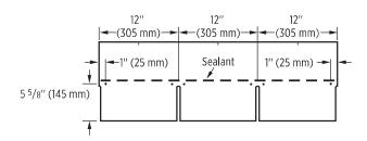
Figure 10-5: Six nails can be used for high wind applications.
