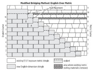
Figure 10-18: Reroofing using standard 12" x 36" shingles over metric shingles.
