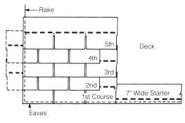
Figure 10-12: Vertical Racking Method.
