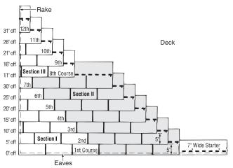
Figure 10-9: Five-Inch, Stepped-Off Diagonal Method.
