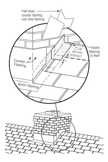
Figure 10-13: Flashing around a chimney.
