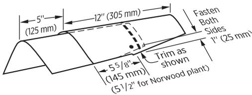
Figure 10-20: Installation of caps along the hips and ridges.
