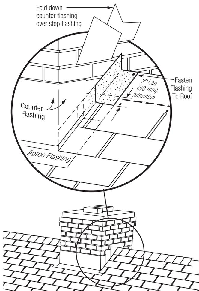
Figure 10-13: Flashing around a chimney.
