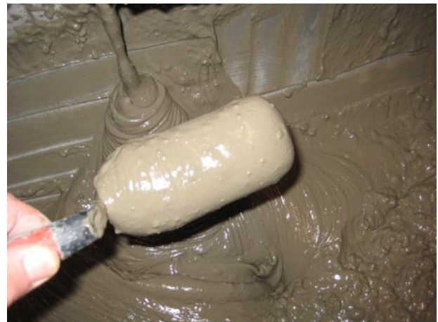
Left: Chunky, undesirable consistency for pumping. Right: Creamy consistency desirable for BentogROUT Injection Pumping.
