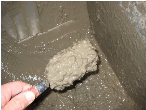
Left: Chunky, undesirable consistency for pumping. Right: Creamy consistency desirable for BentogROUT Injection Pumping.
