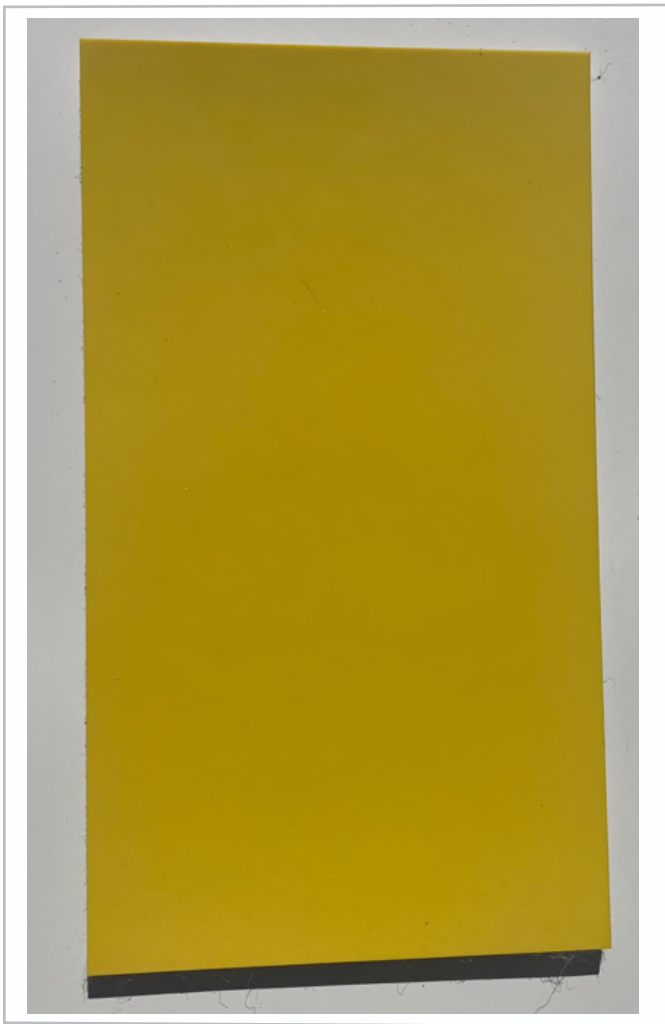
Figure 1: Old COREFLEX/COREFLASH. Lighter yellow appearance. Reinforcement fabric barely visible through PVC layers.
