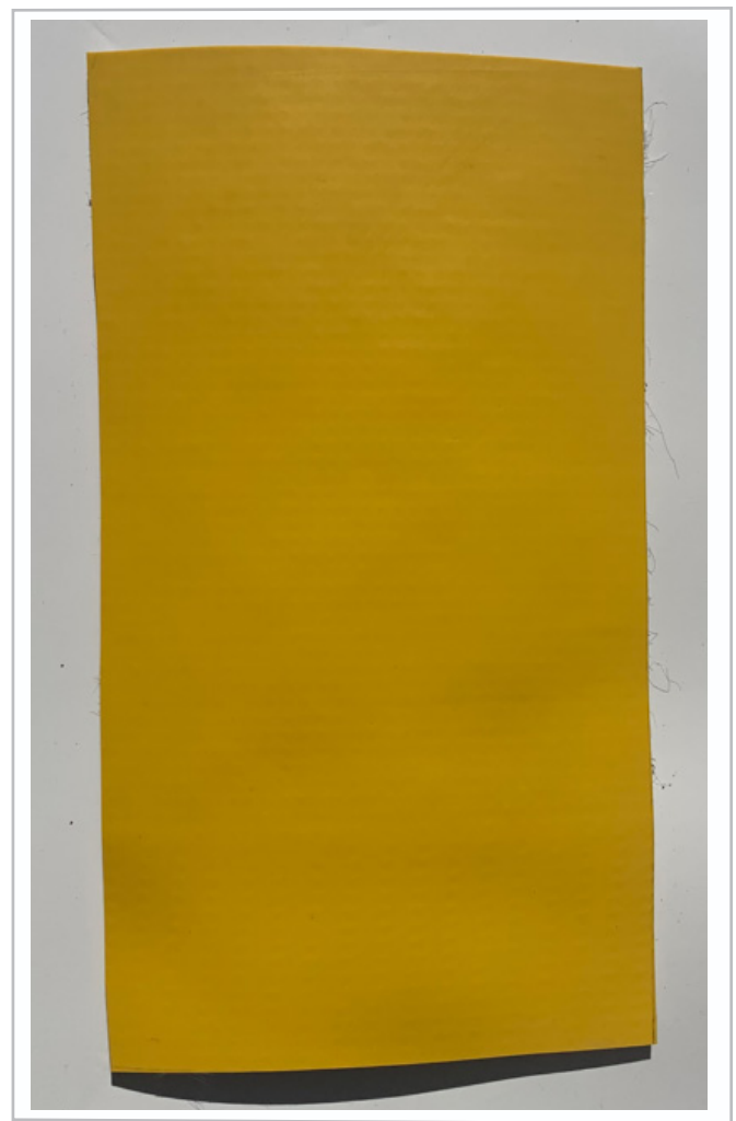
Figure 2: Updated COREFLEX/COREFLASH. Slightly darker yellow appearance with reinforcement scrim pattern visible through PVC layers.
