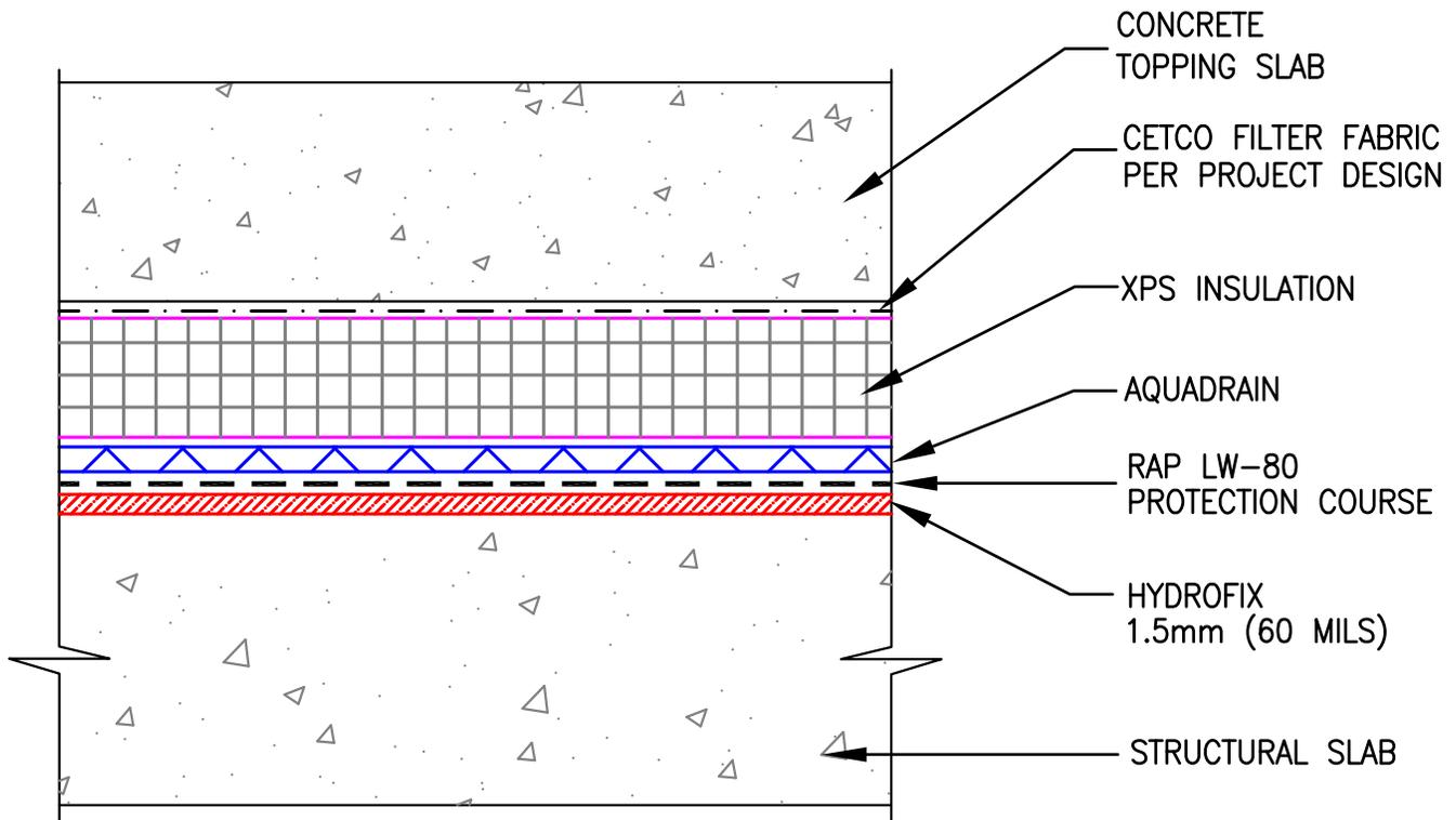
NOTE: CLEAN DECK TO BARE CONCRETE WHERE HYDROFIX IS BEING INSTALLED
