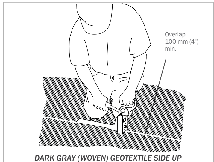
Figure 1.2 – Secure overlaps together with fasteners
