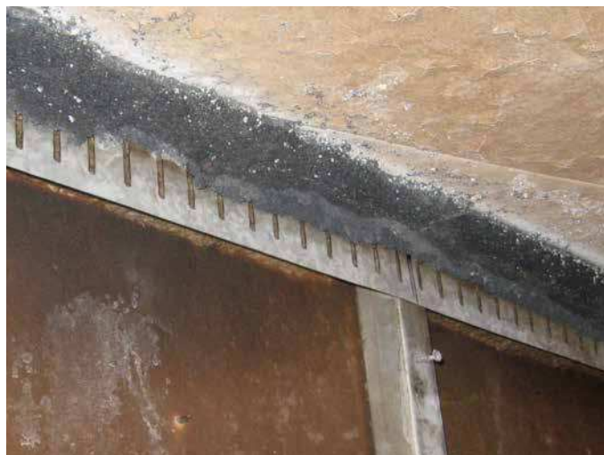
Expanded intumescent strip after fire test
