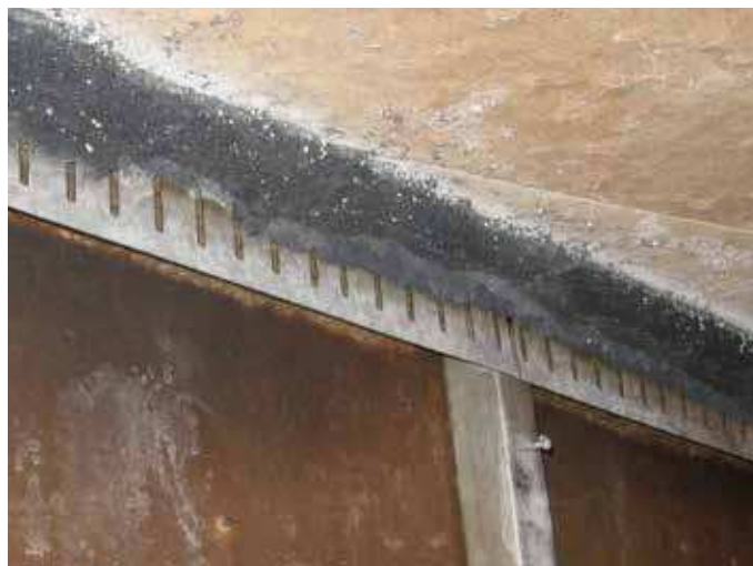
Expanded intumescent strip after fire test
