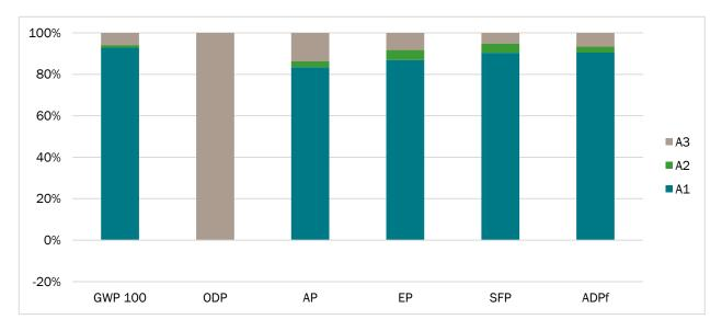
For most impact categories/indicators, the production of raw material inputs accounts for most of the impacts, which is mainly attributed to the steel coil used to create the framing products.
