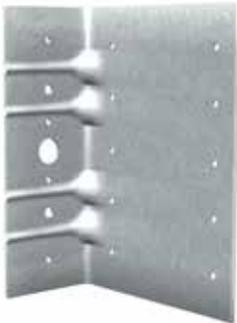
ClarkDietrich EasyClip T-Series™ tall anchor clips are high-performance, cost-effective solutions for knee wall-to-foundation connections, light-duty shearwall-to-foundation connections and truss-to-wall connections. They are designed to resist horizontal, torsional and vertical (uplift) loads.
