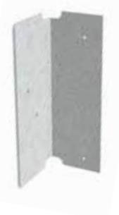
ClarkDietrich EasyClip X-Series™ clip angles are used to secure U-channel to wall studs for lateral bridging. U-channel is passed through the stud knockout and an EasyClip X-Series clip is screw-attached or welded to provide a rigid connection. X-Series clip angles and U-channel should not be used in lateral bridging when stud width exceeds 6".
