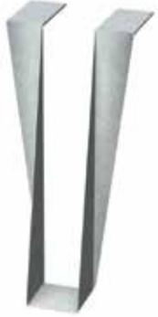
Bridle hangers are commonly used to attach light-gauge C-joists to structural steel beams, wood ledgers or masonry block. Connections can be made with screws, powder-actuated fasteners, drill-in concrete anchors or welding. Single- and double-wide hangers are also available in other widths and depths. The MB hanger can also be sloped to a maximum of 45°. Skew only: MB series can be skewed to a maximum of 45°—maximum allowable download is 62% of table load.
