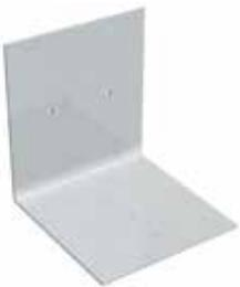
ClarkDietrich aluminum burn clips are used as part of the H-stud area separation wall assembly and are designed to melt when exposed to fire. The clips hold the area separation wall assemblies in place at the floor, roof and truss line between adjacent units. In a fire, the aluminum burn clips on the fire-ridden side of the wall will melt, allowing the wall structure for that side to collapse.
