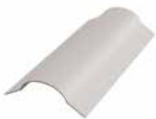
Platinum off-angle nail-on bullnose bead, also known as splayed bullnose or 120°/135° bullnose corner bead, is used to provide a rounded bullnose finish for outside off-angle drywall intersections. Nails or mechanical fasteners are used to secure the bead to the wallboard.
