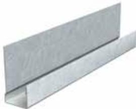
ClarkDietrich metal J-trim is a strong, reveal-type galvanized steel casing that provides maximum corrosion protection and neat finished edges to drywall terminations around door and window openings. It also delivers a clean trim line at intersections or where gypsum panels abut dissimilar surfaces, such as columns and window mullions. Hemmed edges allow quick installation and do not require joint compound.
