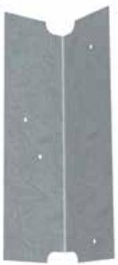
ClarkDietrich EasyClip B-Series™ clip angles are used to secure U-channel to wall studs in back-to-back framing applications and for various miscellaneous rigid connections. The shorter length of the B-Series clip enables it to be installed inside the C-shape. It can also be used to secure lateral bridging on single studs where the clip is preferred to be inside the C-shape. Do not use in lateral bridging when stud width exceeds 6".
