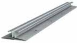
ClarkDietrich expansion joint #40 is a two-piece slip joint that finishes butt ends of adjacent panels in wide or tall walls and ceilings, to allow for multi-directional movement. Ideal for joining dissimilar wall types such as wood framing to CMU and at construction joints. Use where excessive horizontal and vertical movement may occur. Adjustable expansion opening or reveal is 1/4" to 5/8."
