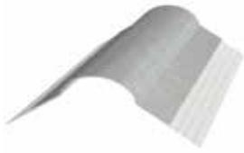
Platinum® tape-on inner cove 90° paper-faced bead provides subtle, rounded inside or inner corners. Inner cove tape-on beads are embedded in joint compound and pressed firmly into place. Excess compound is removed with a drywall knife or wiped clean with a rag.
