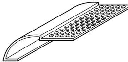
Vinyl Corp. bullnose "J" bead for surface application is designed to be applied after the wallboard is installed. Cover the raw edges of wallboard with a 3/4" radius bead. The perforated flange accepts joint compound or veneer plaster for a flush finish.
