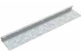
This #66 N short flange galvanized casing bead has the same uses as the #66 expanded flange casing beads associated with select one-coat systems, but it has weep holes for moisture dissipation. Perforated 1-1/4" nailing flange aids attachment and plaster keying.
