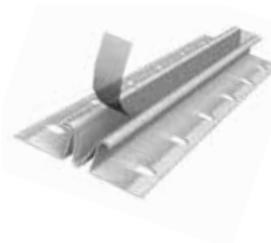
Zinc control joints 38, 50, 75 and 100 are roll-formed from zinc to resist corrosion in both interior and exterior applications with gypsum or Portland cement plaster. An open slot, 1/4" wide and 1/2" deep, is protected with plastic tape that is removed after plaster and finish are completed. Perforated short flanges aid keying and wire attachment to metal lath.
