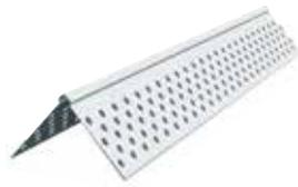
Vinyl corner bead is a rigid, easy-to-apply 90° corner reinforcement that nails or staples into place. Multiple perforations along the flanges enhance bonding. The pronounced nose provides a ground and screed to help achieve precise finishing depth. It's easily cut, dent-resistant, rustproof and maintains shape, with no sharp edges or burrs when field cut.
