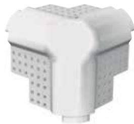
ClarkDietrich 3-way 3/4" bullnose 90° corner caps provide the ideal solution to finish corners quickly and efficiently at 3-way intersections. Features extended tabs for easier alignment and a professional finish. Works well with both metal and vinyl bullnose corner beads, eliminating the need for special corner bead applications and mitering.
