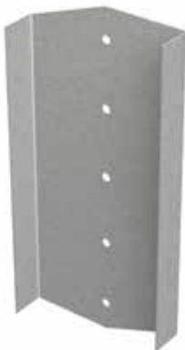
EasyClip QuickTwist™ web stiffeners are used to provide reinforcement of joist webs to prevent crippling. Web reinforcement is often required by design to enhance the load capacity of joists. The unique design of QuickTwist allows the installer to insert the stiffener on the inside of the joist *after* the joist is installed. This stiffener eliminates the need to pre-insert traditional web stiffeners prior to joist installation.
