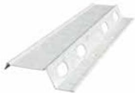
Made of 25 gauge steel, RC-1 Pro is used as a cross-furring member for resilient attachment of gypsum. Knurled face makes wallboard application easier.
