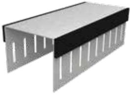
Profile with two slotted legs with fire stop on both sides. Composite fire stop/framing for use in fire-rated wall assemblies. Provides 100% unencumbered joint protection. Accommodates up to 1-1/2" overall movement with UL 2019 Level III Certification. Minimum CP60 coating. Legs with slots spaced 1" o.c. for positive attachment of studs per listed assemblies in UL Fire Resistance Directory.
