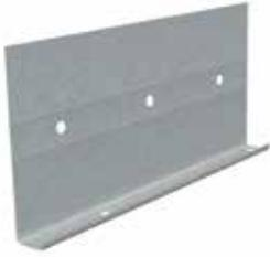
J-weep high-back plaster stop is a J-shaped square-nosed trim manufactured from 26 gauge galvanized steel. Punched weep holes allow for use as a sill weep screed or screed and trim around wall openings. Squared bends accommodate 1" rigid insulation and 3/8" one-coat stucco applications.
