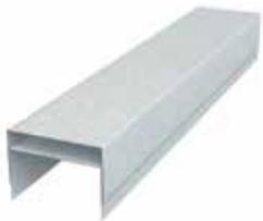
ClarkDietrich DoubleTrack™ system is a two-piece assembly that accommodates deflection of exterior curtain walls. A custom-made deep leg outer track is installed to the underside of the floor deck. A wall assembly is constructed on the floor and slid into place, with a “gap” at the top for deflection. DoubleTrack deflection assemblies cannot be used in axial load-bearing stud conditions or above continuous window spandrels.
