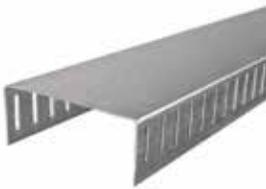
MaxTrak® is a head-of-wall deflection track that is used for framing exterior curtain walls and nonload-bearing interior walls where vertical deflection occurs—and serves as a connecting member that isolates the cold-formed steel framing system from the movement of the primary structure.
