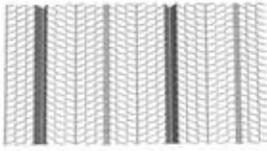
ClarkDietrich 3/8" high rib lath is the most rigid of all laths and provides the added support required when framing is more than 16" o.c. but does not exceed 24" o.c. Commonly used for soffits and ceilings under steel or wood joist construction and metal-reinforced concrete floors. 3/8" V-shaped ribs run the length of the sheet at 3-7/8" intervals and inverted 3/16" intermediate ribs.
