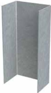
ClarkDietrich web stiffeners are used to provide reinforcement of joist webs to prevent crippling. Web reinforcement is often required by design to enhance the load capacity of joists. When installing between the joist flanges, a web stiffener must be installed by sliding it in from the end of the joist.
