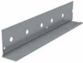
ClarkDietrich metal L-trim provides a clean finished edge at door and window openings or when wallboard abuts dissimilar surfaces, such as suspended ceilings, beams, plaster, masonry and concrete. Installed after the gypsum panels are already in place—unlike Spackle J which must be installed during gypsum panel installation—L-trim is easily attached with screws or nails. A hemmed front flange provides rigidity.
