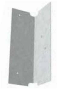
ClarkDietrich EasyClip X-Series™ clip angles are used to secure U-channel to wall studs for lateral bridging. U-Channel is passed through the stud knockout and an EasyClip X-Series clip is screw-attached or welded to provide a rigid connection. X-Series clip angles and U-channel should not be used in lateral bridging when stud width exceeds 6."
