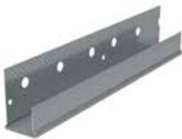
ClarkDietrich U-trim, or Spackle J, provides maximum protection and clean finished edges on gypsum panels around door and window openings, and when wallboard abuts dissimilar surfaces, such as suspended ceilings, beams, plaster, masonry and concrete. It's easily installed by sliding trim over the edge of the board and nailing/ screwing through the knurled (long) flange—which also enhances compound adhesion.
