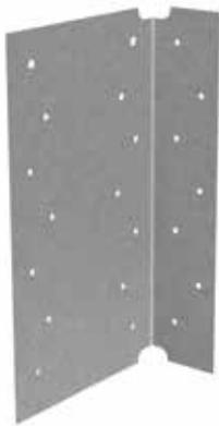
ClarkDietrich EasyClip™ E-Series™ support clips are used for rigid standoff connections. The 4" wide leg provides extra length to achieve standoff connections up to 3". These support clips are commonly used in bypass wall conditions, solid blocking attachments in joist framing, and to secure rafter framing to the primary structure. EasyClip E-Series support clips are prepunched for faster and more accurate fastener placement.
