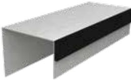
Profile with two solid legs with fire stop on one side. Composite fire stop/framing for use in up to three-hour fire-rated shaft wall assemblies. Provides 100% unencumbered joint protection. Accommodates up to 1-1/2" overall movement with UL 2019 Level III Certification. Minimum CP60 coating. One leg (front) having intumescent per listed assemblies in UL Fire Resistance Directory.
