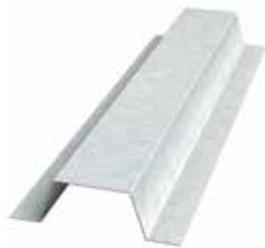
ClarkDietrich heavy-duty furring channel is a high-performance framing component used in ceiling, exterior wall and roof applications. With two standard depths—7/8" and 1-1/2"—heavy-duty furring channel provides greater resistance to deflection and bending. In roof applications, heavy-duty furring is used as purlins to provide connection points for roof sheathing.
