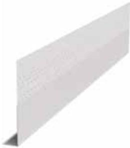
Platinum L-trims are used to finish the ends of wallboard where it abuts dissimilar surfaces, such as suspended ceilings, beams, plaster, masonry or untrimmed door and window jambs. Applied in the same manner as all other tape-on beads—joint compound embeds the paper-faced bead to the wallboard paper.
