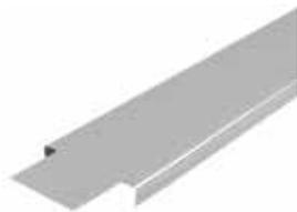
Katz™ bridging maintains accurate member spacing to prevent bowing or flexing of nonload-bearing framing. It can also be used as backing between studs in areas where cabinets or fixtures are to be attached. Use standard 24" o.c. frame spacing.
