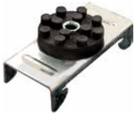
The RSIC-1® resilient sound isolation clip is used in conjunction with drywall furring channel to fasten gypsum wallboard to various wall and floor-ceiling designs and applications, while simultaneously providing acoustical separation (decoupling). This significantly reduces the amount of impact and sound that filters from surrounding rooms—reducing the noise transfer by 75 to 100%.
