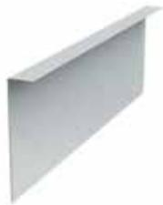
ClarkDietrich L-headers are prefabricated, light-gauge 90° L-sections that are used in load-bearing wall framing. They slide easily into place and eliminate the labor-intensive process of built-up field-assembled headers. Install as single, one header one side, or double, two headers, one on both sides.
