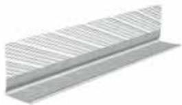
Our veneer trims are L-shaped trims designed for use at junctions of veneer gypsum base with rough concrete or masonry ceilings. Sized to fit standard gypsum plaster bases, the trim with 3/32" grounds is for two-coat veneer, and the trim with 1/16" grounds is for one-coat veneer plaster.
