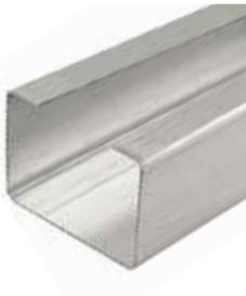
Headers are prepunched, and pre-cut to the length specified on your order. Header depth is 1/8" narrower than jamb depth to accommodate fit into HDSC Clip. Header lengths should be ordered 1/2" shorter to fit inside clips.
