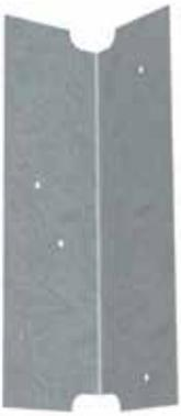
ClarkDietrich EasyClip B-Series™ clip angles are used to secure U-channel to wall studs in back-to-back framing applications and for various miscellaneous rigid connections. The shorter length of the B-Series clip enables it to be installed inside the C-shape. It can also be used to secure lateral bridging on single studs where the clip is preferred to be inside the C-shape. Do not use in lateral bridging when stud width exceeds 6".
