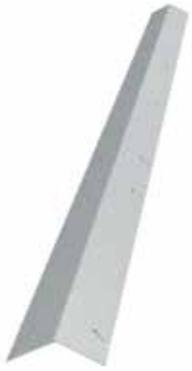
ClarkDietrich TradeReady® Spazzer® 5400 spacer bar is a galvanized steel spacer and bridging bar, engineered to facilitate the rapid erection of exterior curtain wall framing, load-bearing walls and high interior partitions constructed of structural studs. Proprietary prepunched slots provide excellent torsional and lateral stud restraint.
