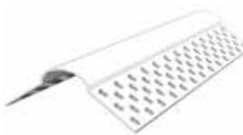
ClarkDietrich vinyl bullnose splayed corner bead is used to finish off-angle interior corners from 120–135° when a rounded “bullnose” look is desired. This durable trim product is dent-resistant, rustproof and easily finished. Multiple elongated perforations along both flanges enhance joint compound bond.
