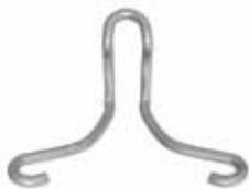
In a ceiling assembly, furring channel clips can be used to suspend U-channel from the overhead structure. Drywall furring channel is commonly clipped or wire-tied perpendicular to the underside of the U-channel at appropriate intervals for screw-attaching drywall.
