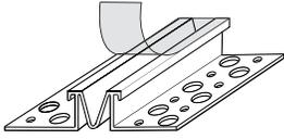
Used to provide stress relief and assist in controlling cracking in large areas of walls and ceilings, control joints with removable tape protect the deep “V” expansion slot during construction. Specially designed Connector Clips are provided for alignment and base for sealants. Recommended for smooth finishes.
