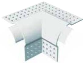
ClarkDietrich vinyl 2-way 3/4" corner caps provide the ideal component to transition bullnose corner beads to a crisp finish where inside corners intersect at 90°. Examples of applications include windows, closets, doorways, skylights, etc. Easy to install, this component provides a cost-effective alternative to time-consuming mitering of corners.
