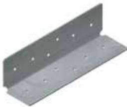
SwiftClip™ LS-Series™ support clips are used in multiple construction projects, specifically in conjunction with studs and track. The L-shaped clips fit between the stud flanges, so that shorter length clips do not need to be ordered. These labor time-savers include prepunched holes for quicker screw attachments, and are punched to accommodate for U-channel lateral bracing connections.
