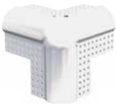
ClarkDietrich 3-way 3/4" bullnose 90° corner caps provide the ideal solution to finish corners quickly and efficiently at 3-way intersections. Features extended tabs for easier alignment and a professional finish. Works well with both metal and vinyl bullnose corner beads, eliminating the need for special corner bead applications and mitering.
