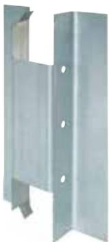
For use with the FastBack® backing system, the FastBack backing clip conceals fasteners on the face of the product. Rotate the FastBack clip over the flange of the stud until it sits flush. Then fasten into place using drywall screws in the pre-drilled holes.
