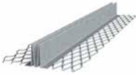
Double-V, sometimes called M-Type control joints, relieves the stresses of basic expansion and contraction associated with inherent shrinkage during stucco curing and general thermal changes. Resists corrosion, plus expanded flanges allow for proper keying and easy installation. Ground heights include 3/8" for thin-coat plaster and 1/2", 3/4" and 7/8" for conventional plaster.
