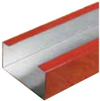
Unpunched headers are pre-cut to the length specified on your order. Header depth is 1/8" narrower than jamb depth to accommodate fit into Drop 'N Lock clip. Header lengths should be ordered 1/2" shorter to fit inside our Drop 'N Lock clips. RedHeader RO Extra-Duty headers have a longer 3-1/2" flange for wider spans.
