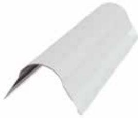
Platinum® 3/4" tape-on bullnose corner bead is used to create a smooth, rounded look to standard drywall corners. It adds contemporary styling and a sense of openness to any room. Apply in the same manner as all other tape-on beads. Gypsum boards must be cut back 3/4" to accommodate the bullnose and ensure a flush fit.
