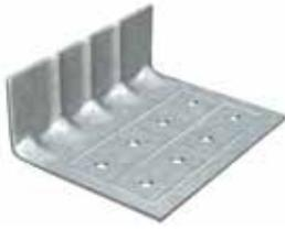
ClarkDietrich's Uni-Clip™ end clip is a universal framing clip used to attach and support numerous rigid framing conditions. The Uni-Clip framing clip has a stiffened corner that provides superior design values and is installed easily with screws or powder-actuated fasteners. This clip is ideal for most rigid connections, including shear, tension and two-axis loading.
