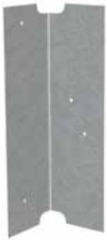
ClarkDietrich EasyClip U-Series clip angles are used to secure U-channel to wall studs for lateral bridging or for miscellaneous rigid connections. U-channel is passed through the stud knockout and an EasyClip U-Series clip is screw-attached or welded to provide a rigid connection. These clips are prepunched for faster, more accurate fastener placement. Do not use in bridging applications when the stud width exceeds 6."
