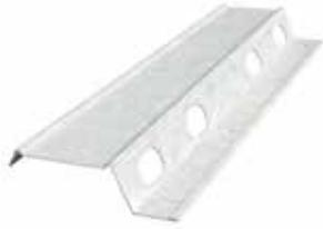
Made of 22mil steel, RC-1 ProPlus is used as a cross-furring member for resilient attachment of gypsum. Knurled face makes wallboard application easier.
