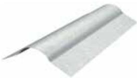
ClarkDietrich splayed or off-angle bullnose is used to create a smooth rounded look at 135° corners. Bullnose adds contemporary styling, but also performs with corrosion protection and durability. Available with a galvanized finish conforming to ASTM C1047 or prime-painted surface for shadow-free finishing.
