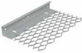
Designed for use with select, tested and approved one-coat plaster systems, this version of the #66 expanded flange casing bead includes weep holes for moisture dissipation. Expanded flange is 3-1/8" wide to aid plaster keying.
