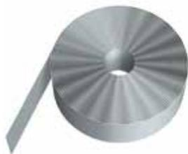
ClarkDietrich diagonal tension strapping, combined with gusset plate components, provides shearwall (racking restraint) for light-gauge, load-bearing framing under wind and seismic loads. Straps should be positioned diagonally in an X-configuration from the bottom to top track—on both sides of the wall. At a minimum, double studs at the ends of the X-brace serve as compression studs, which must be anchored to the foundation.
