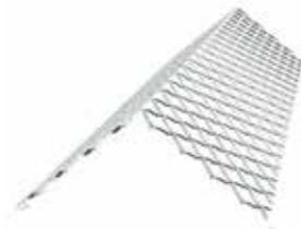
Cornerite™ metal lath angle is used to reinforce all inside lath corners to reduce corner cracking. Formed from finished edge strip lath, it's bent lengthwise to a 100° angle to ensure a snug fit into 90° corners. It's commonly used when walls meet walls or ceilings, over inner angles of masonry construction. Cornerite is produced to ASTM C1063 standards.
