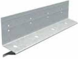
F.H.A.7 foundation weep screed protects the stop edges of stucco and exterior insulated finish system materials at the sill plate. Commonly referred to as F.H.A. screed, it meets all pertinent IBC/IRC requirements as part of a drainage system for exterior stucco applications.
