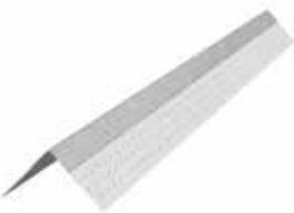
Platinum tape-on inside 90° paper-faced corner bead provides very straight and precise inside corners. The rigid, steel-reinforced inside corners provide a durable guide to achieve exceptionally straight and sharp inside corners. Embed in joint compound and press firmly into place. Remove excess compound with a drywall knife.
