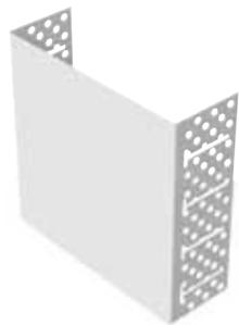
Vinyl partition end caps quickly finish doorways, knee walls and wall ends, providing a finished face. Designed with a special factory punched "T" slotted flange, they can be easily cut to form arches or curves. Instead of installing two corner beads, you install a single piece, using less compound. Easy to cut, rustproof and dent-resistant.
