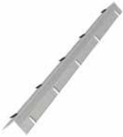
The TradeReady® Spazzer® 9200 bar is a pre-notched, 20 gauge, galvanized steel spacer and bridging bar. It facilitates rapid erection of studs into a rigid, accurately laid out gridwork that has excellent resistance to stud rotation and displacement. Hanging drywall is also faster and easier because the Spazzer 9200 bar eliminates the bow that often occurs in tall interior studs.
