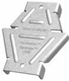
The ClarkDietrich FastBridge™ Clip is used to secure 1-1/2" U-channel [Cold Rolled Channel (CRC)] to structural wall studs when used in load-bearing or curtain wall applications. The wall stud friction fit design allows for as little as one screw for the connection to the U-channel. Do not use in studs over 8" wide.
