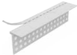
ClarkDietrich Vinyl Rip Bead™ L-trim produces an exceptional finish at intersection of gypsum panels to ceiling grid, window returns and dissimilar wall types. A tear-away strip provides a protective edge and guide for drywall finishing knives. Once joint compound is applied, finished and painted, remove the tear-away strip to form a crisp, clean edge.
