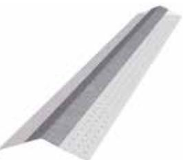
Platinum off-angle tape-on 120/135° inside (or reverse splayed) bead is used to achieve a crisp, clean, straight-finished inside off-angle drywall finish. This bead can be used for inside corner angles between 120° and 135°. As with all tape-on beads, off-angle bead is applied using joint compound. No mechanical fasteners are required.
