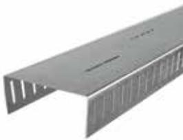
MaxTrak 2D is a head-of-wall deflection track that is used for framing exterior curtain walls and nonload-bearing interior walls where vertical deflection and horizontal drift occurs—and serves as a connecting member that isolates the cold-formed steel framing system from the movement of the primary structure.
