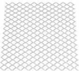
ClarkDietrich utility lath is a superior multipurpose expanded steel product widely used for ceramic tile and floor leveling, and for plaster and stucco repair and remodel. It is available in both the Junior™ mesh style as well as self-furring dimpled product. The self-furring product is manufactured with 1/4" deep dimples that raise the mesh away from solid surfaces for superior mechanical bonding.
