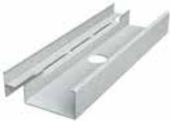
Engineered to maintain shaftwall integrity, ClarkDietrich CT cavity shaftwall studs are punched with 1" circular knockouts at 12" o.c. for easy installation of conduit or other mechanical service lines.
