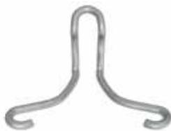
ClarkDietrich metal furring channel clips are made of galvanized wire and used to attach metal furring channels to 1-1/2" U-channels in ceiling gridwork. Clips must be installed on alternating sides of the 1-1/2" channels. Use tie wire when clips cannot be alternated. Clips should only be used when single-layer gypsum or single-layer veneer plaster base is used.
