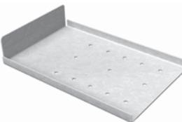
ClarkDietrich's Extended Uni-Clip™ rigid framing clip is used to attach exterior wall studs to the structure of the building. Designed to resist horizontal and vertical loads, the extended rigid clips install easily with screws, powder-actuated fasteners, or welds. This clip is ideal for all medium and large standoff conditions.
