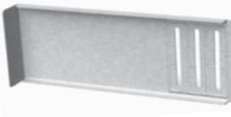
ClarkDietrich Extended FastClip™ deflection clips are used to attach exterior curtain wall studs to the building structure and provide for vertical building movement independent of the cold-formed steel framing. Clips are ideal for medium to larger standoff conditions. Install quickly with screws, welds or powder-actuated fasteners, and they provide adjustable standoff to ensure a plumb wall plane.
