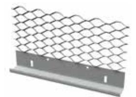
ClarkDietrich #66 expanded flange casing beads are used as a plaster stop, an exposed trim around wall openings, and at junctions or intersections of plaster and other wall or ceiling finishes. Extra-long expanded flange for tie-on applications. Short 90° return flange at plaster surface ensures a neat finish.
