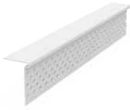
ClarkDietrich L-stop bead creates a clean detail at gypsum panel terminations into doors, windows and ceilings. Easily attaches with nails, screws or staples to studs through bead flange. Multiple perforations along 1-1/4" flange and raised shoulder enhance strong compound adhesion and provide for a flush finish. Rustproof, dent-resistant and easy to field cut without distorting profile or leaving sharp edges and burrs.
