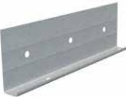
1-3/8" J-weep low-back is commonly used as a stop around door and window openings or in areas where stucco or E.I.F.S. terminations abut dissimilar wall types. Nail, screw or staple-attach to the frame or sheathing, then foam insulation, cement board or metal lath can be installed over it. The protruding ridge of the metal must extend beyond the plane of overlaid materials.
