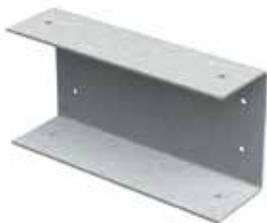
The HDSC header bracket is the perfect complement to the HDS Framing System. This simple, yet innovative header bracket turns a two-person curtain wall header installation into a one-person job. This unique, prepunched clip also eliminates surface head fastener buildup that can create finishing challenges.
