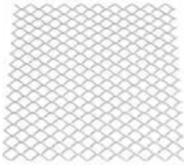
ClarkDietrich Junior™ diamond mesh lath is used as a substrate for Portland cement or gypsum plaster stucco on either interior or exterior walls, ceilings, soffit and fascia surfaces, and can be used under ceramic tile in wall, ceiling and floor applications. It's useful in all general-purpose applications and is the best lath available for ornamental work and contoured surfaces, as well as spray-applied fireproofing.
