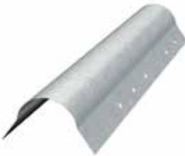
ClarkDietrich bullnose corner bead is used to create a smooth, rounded look to standard drywall corners. Of rugged steel construction, bullnose 90° corner bead is designed for superior compound adhesion. Just nail, screw or staple in place. Available with a galvanized finish meeting ASTM C1047 or with a prime-painted surface for shadow-free finishing.
