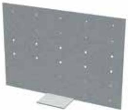
The H-Series™ universal header hanger is used to connect box headers to jambs, or beams to columns, and transfer large vertical loads. This universal hanger is designed so one part can be used for either side of the connection. The hanger also features a support tab for proper alignment and easy installation.
