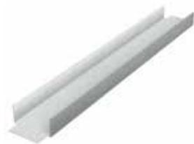
ClarkDietrich Katz™ blocking is specifically manufactured to ladder frame between parallel framing members and provide for the attachment of the top of the interior nonstructural walls when trusses or floor joists run parallel to the walls. Katz blocks are secured to the floor joists or roof trusses with screws or nails.
