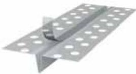
ClarkDietrich 093 zinc control joint is applied between abutting gypsum panels, and is used to relieve stresses of expansion and contraction of drywall and veneer plaster systems in large ceiling and wall expanses over 30' in length. It's typically installed from door header to ceiling, from floor to ceiling in long partition runs, and from wall to wall in large ceiling areas—and for interior or exterior applications.
