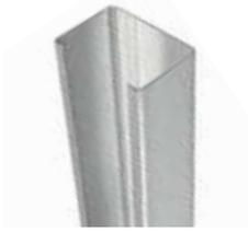
As part of the RedHeader RO system, the jamb eliminates capped members, allowing drywall screws to drive through only one thickness of material. Plus, the open jamb does not require pre-insulating. RedHeader RO Extra-Duty jambs have a longer 3-1/2" flange for wider spans.
