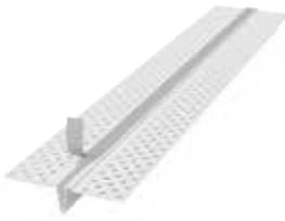
Vinyl 093 control joint is applied between abutting gypsum panels to relieve stresses of expansion and contraction of drywall in large ceiling and wall expanses over 30'. Typically installed from door header to ceiling, from floor to ceiling in long partition runs, and from wall to wall in large ceiling areas. Remove plastic tape (protects 1/4" opening x 7/16" deep reveal) after compound is applied and finished.
