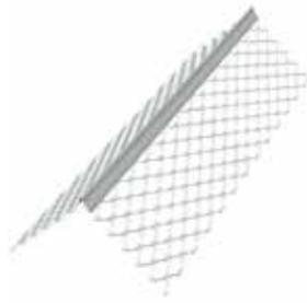
ClarkDietrich 1A expanded flange corner bead is used to provide strong corner reinforcement for conventional plaster applications. A solid metal nose provides a straight, rigid ground for screeding, and the 2-7/8" or 3" flanges can be flexed easily over irregular, uneven surfaces. Plaster keys near the solid nose provide increased reinforcement where needed and ensure straight corners.
