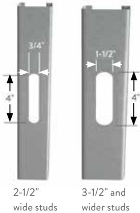
ClarkDietrich light-gauge C-studs for axial load-bearing and curtain wall framing are prepunched with knockouts at regular intervals. These punchouts are specifically designed to allow for rapid installation of pipes, electrical conduit and wall bridging.
