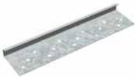
ClarkDietrich #66 N short flange casing beads are used as plaster stops, as exposed trim around wall openings and junctions, or at intersections of plaster and other wall or ceiling finishes. Perforated 1-1/4" nailing flange aids attachment and plaster keying. When used in conjunction with lath, the 66 N is installed under the lath.
