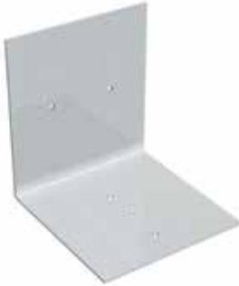
ClarkDietrich aluminum burn clips are used as part of the H-stud area separation wall assembly and are designed to melt when exposed to fire. The clips hold the area separation wall assembly in place at the floor, roof and truss line between adjacent units. In a fire, the aluminum burn clips on the fire-ridden side of the wall will melt, allowing the wall structure for that side to collapse.
