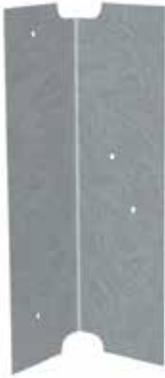
ClarkDietrich EasyClip™ U-Series™ clip angles are used to secure U-channel to wall studs for lateral bridging or for miscellaneous rigid connections. U-channel is passed through the stud knockout and an EasyClip U-Series clip is screw-attached or welded to provide a rigid connection. These clips are prepunched for faster, more accurate fastener placement. Do not use in bridging applications when the stud width exceeds 6".
