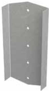
EasyClip™ QuickTwist™ web stiffeners are used to provide reinforcement of joist webs to prevent crippling. Web reinforcement is often required by design to enhance the load capacity of joists. The unique design of QuickTwist allows the installer to insert the stiffener on the inside of the joist *after* the joist is installed. This stiffener eliminates the need to pre-insert traditional web stiffeners prior to joist installation. The one-piece assembly is easily rotated in-place for a tight fit.
