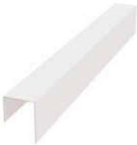
ClarkDietrich vinyl J-bead provides a finished edge at gypsum board stops around door and window openings and at ceiling intersections. Requires no joint compound. Rigid vinyl is not a thermal transmitter and helps stop condensation where gypsum board terminates at exterior metal surfaces, such as window frames and mullions. Rustproof and dent-resistant.
