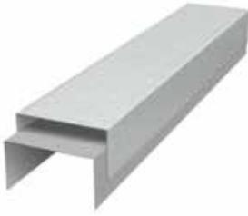
ClarkDietrich DoubleTrack™ system is a two-piece top track assembly that allows for the deflection of floor beams or floor decks along interior partitions. A custom-made long leg outer track is installed to the underside of the floor deck. A wall assembly is constructed on the floor then slid into place. The wall assembly is designed to allow a “gap” at the top for deflection.
