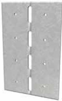
The ClarkDietrich field skewable TradeReady® rim track splice plate provides an easy and efficient method for splicing TradeReady rim. This prepunched plate is also ideal for connecting and reinforcing the rim at bay or bow window details. The center of the plate allows for easy one-time field bending from 0° to 135°.
