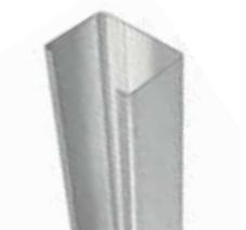
As part of the RedHeader RO system, the jamb eliminates capped members, allowing drywall screws to drive through only one thickness of material. Plus, the open jamb does not require pre-insulating.
