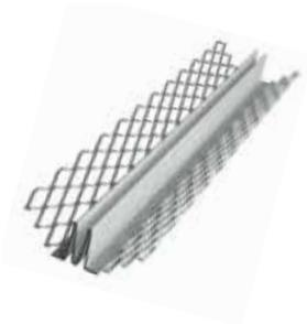
ClarkDietrich Corner Master™ #30 inside corner control joint is designed to provide stress relief at plaster wall inside corner intersections, by absorbing movement and controlling cracking. It has expanded flanges pre-formed at 90° for a flush fit at inside corners. Ground heights offered aid plaster keying and result in a clean, straight finish. Manufactured from galvanized steel for corrosion protection.
