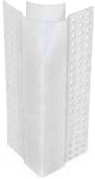
ClarkDietrich bullnose to 90° transition caps simplify installation of baseboard or crown molding corners into 3/4" bullnose systems. Quick and easy to install, they eliminate corner gaps and the need for time-consuming caulking and filling. Use with metal, vinyl or paper-faced 3/4" bullnose corner bead for transition onto baseboard or crown molding up to 4-1/2" wide.
