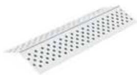
ClarkDietrich 120/135° corner or splayed bead is used to finish off-angle interior corners from 120–135°. Designed to provide straight, rustproof, dent-resistant corners, its flexibility allows a flush fit on many unusual outside wallboard intersections. Multiple perforations along the flanges enhance joint compound bonding.
