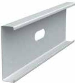
ClarkDietrich C-joist components provide an economical, lightweight alternative to open web trusses, bar joists, engineered lumber, cast-in-place or hollow core floor assemblies. Plus, they're pre-cut to save time. Depending on loads and spans, C-joists are typically spaced at 12", 16", 19.2" or 24" o.c. Joist-to-girder attachments are normally supported with joist hangers, EasyClip E-Series™ or S-Series™ support clips. Web stiffeners may be required at supports and other point loads.
