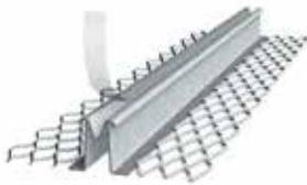
A general-purpose control joint offering exceptional expansion control for plastered walls and ceilings, the double-J expansion control joint has a 5/16" reveal and rolled outer edges that allow effective plaster bonding. This helps prevent visible separation cracks. The applied plastic tape keeps the reveal clean and is removed easily after finish application.
