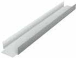
The third component of the TradeReady® Floor System, TradeReady structural blocking is pre-cut to fit securely between the underside of the floor joists to prevent joist rotation. Prepunched for quick attachment, it's an economical alternative to cross bracing, X-bracing or strapping. For easy attachment, install continuous row of blocking every 8' o.c. maximum, and staggered.
