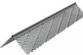
ClarkDietrich Mini-Bead™ 800 and 900 are fine-mesh corner beads used to provide corner reinforcement. Mini-Bead 800 has 1/16" grounds for one-coat veneer plaster and 90 keys per linear foot for excellent bonding and strong corners. Mini-Bead 900 has 3/32" grounds for two-coat veneer plaster systems.
