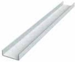
ClarkDietrich U-channel, combined with EasyClip™ clip angles (U-Series™) and screws, is one of the most common bridging methods used to provide resistance to stud rotation and minor axis bending under wind and axial loads. 1-1/2" U-channel is passed through the stud knockout and secured. Lateral bracing is typically installed at a maximum of 48" o.c., but consult ClarkDietrich's Technical Design Guide for proper spacing.
