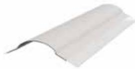
Platinum off-angle bullnose tape-on bead (also known as splayed bullnose or 120°/135° bullnose corner bead), is used to provide a rounded, bullnose finish for off-angle drywall intersections. It is applied in the same manner as 90° paper bead. Gypsum board must be cut back 3/4" to accommodate the bullnose and ensure a flush fit.
