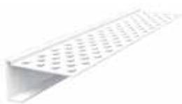
Mudable J-bead is used to cover and protect exposed ends of gypsum panels that abut other substrates like masonry, glass and metal frames. Raised shoulder and extensive perforations along flange ensure excellent finishing compound adhesion and flush finish. Moisture- and thermal-resistant properties make this ideal around bathtubs, showers, windows and skylights. Rustproof, dent-resistant, easy to cut and install.
