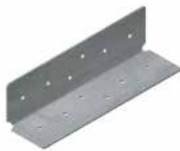
SwiftClip LS-Series™ support clips are used in multiple construction projects, specifically in conjunction with studs and track. The L-shaped clips fit between the stud flanges, so that shorter length clips do not need to be ordered. These labor time-savers include prepunched holes for quicker screw attachments, and are punched to accommodate for U-channel lateral bracing connections.
