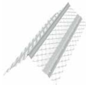
ClarkDietrich Double-X™ or 2A galvanized corner bead, provides additional rigidity for reinforcing plaster corners. The Double-X is an ideal choice for corners in high-traffic areas. Combination of expanded flanges and pronounced bead nose ensures effective corner alignment and efficient plaster keying from edge to nose.
