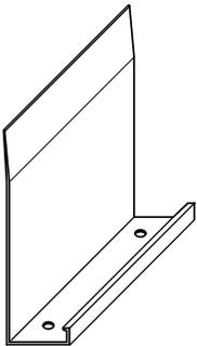
Foundation weep screed acts as a stop, and is designed with an unperforated flange, allowing moisture removal from stucco installations on frame construction at the foundation line.
