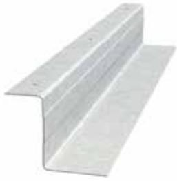
ClarkDietrich Z-furring is used to furr out interior masonry or poured concrete wall substrates and to support rigid polystyrene, mineral, or fiberglass batt insulation while providing a uniform plane for gypsum panel attachment. Z-furring should be installed vertically with the 3/4" flange against the substrate. The type of fastener and spacing will vary based on application. Install gypsum wallboard parallel or perpendicular to Z-furring.
