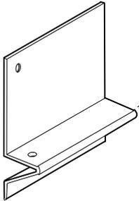
Designed to relieve moisture from stucco/stone and act as a stop. Install on frame construction where stucco/stone and foundation walls meet. Shown here is standard weep screed.
