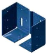
Prepunched slots allow for vertical field adjustments before fully attaching the clip to the RedHeader RO jamb stud. The narrower header and clip width reduce material buildup that pushes the gypsum board out, eliminating additional corner bead and taping costs.
