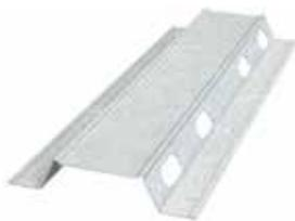
Made of 22mil steel to provide a stiffer resilient channel, RC-2 ProPlus heavy-duty double-leg resilient channel is typically used for ceiling applications with multiple layers of gypsum board. It is used as a cross-furring member for resilient attachment of gypsum. Knurled face makes wallboard application easier.
