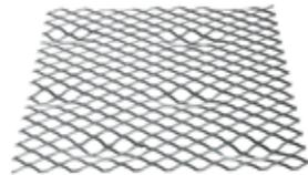
ClarkDietrich self-furring lath is manufactured with approximately 1/4" deep dimples that raise diamond mesh away from solid surfaces to enable thorough plaster or stucco penetration into and behind the lath for superior mechanical bonding. The dimples are spaced every 4-6" over the rectangular sheet. This lath is to be used in manufactured stone installations, per ASTM 1780.
