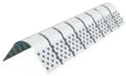
ClarkDietrich vinyl bullnose archway corner bead provides a rounded, contemporary look to archways, curves or just about any radius. Notched flanges enable it to be arched to an inside or outside radius. Secure each tab on the archway bead with adhesive or staples before application of joint compound.
