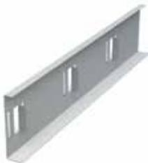
Another major component of the TradeReady floor system, the standard 16'-long rim drastically reduces framing time and effort. Rims have pre-formed, prepunched attachment tabs at 12", 16", 19.2" or 24" o.c. spacing to eliminate layout time—and ensure fast, proper fastener placement. Embossed stiffening ribs on each side of the tabs provide additional reinforcement, for a significant reduction of web stiffeners (squash blocks) and support clips in a majority of applications.
