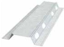
Made of 25 gauge steel, RC-2 Pro double-leg resilient channel is typically used for ceiling applications. It is used as a cross-furring member for resilient attachment of gypsum. Knurled face makes wallboard application easier.
