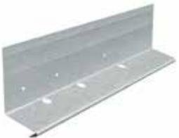
7/8" sill screed is a similar profile to the F.H.A.7 foundation weep screed except the bottom flange has been cut back to allow trowel access for cleaning excess material and trimming of the vapor barrier. It offers impact and splash protection, and meets all other applicable codes with respect to 3-1/2" nailing flange, 26 gauge galvanized steel and 7/8" ground.
