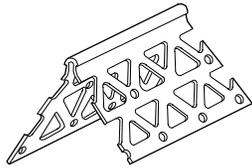
Vinyl Corp. #1 corner bead provides hard-to-damage, rustproof, straight corners, and is easily curved for smooth arches. A heavier version of our #1 corner bead, the #2 corner bead also has wider flanges. #2 corner beads should be used where a more durable corner is required.
