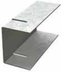
A ClarkDietrich Slide Clip™ is used to attach exterior curtain wall studs to the building structure and provide for vertical building movement independent of the cold-formed steel framing. Slide clips are used in bypass framing situations and are normally welded or otherwise fastened to the vertical leg of a structural angle at the floor or roof edge.
