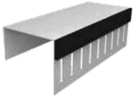
Profile with one slotted leg and one solid leg with fire stop on slotted side. Composite fire stop/framing for use in fire-rated wall assemblies. Provides 100% unencumbered joint protection. Accommodates up to 1-1/2" overall movement with UL 2019 Level III Certification. Minimum CP60 coating. One leg with slots spaced 1" o.c. for positive attachment of studs per listed assemblies in UL Fire Resistance Directory.
