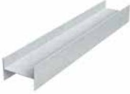
ClarkDietrich H-studs are 2" wide vertical members used to secure two 1" thick pieces of gypsum shaftliner in area separation wall assemblies. H-studs are inserted into C-runners and slid over gypsum panel liner edges, repeating until the desired wall length is achieved. Once the wall is plumbed, it is secured with aluminum burn clips.
