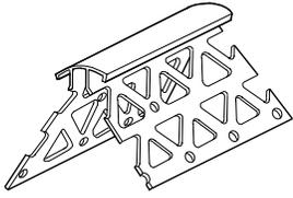
Designed for use in applications such as schools and hospitals, Vinyl Corp.'s #1B 3/4" bullnose corner bead provides hard-to-damage, rustproof, soft corners. The #2B bullnose corner bead is a heavier version that is appropriate for applications where a more durable corner is required.
