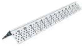
ClarkDietrich vinyl archway corner bead fits almost any arch, curve or radius to provide rigid corner and edge protection. The notched single flange adapts to virtually any radius condition. Multiple perforations along flanges and notches enhance joint compound bonding. In addition to nails or staples, use an adhesive to secure arch tabs to gypsum board.
