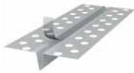
ClarkDietrich 093 zinc control joint is applied between abutting gypsum panels to relieve stresses of expansion and contraction of drywall and veneer plaster systems in wall expanses over 30', and ceiling areas exceeding 2,500 square feet. It's installed from door header to ceiling, from floor to ceiling in long partition runs, and from wall to wall in large ceiling areas or in areas where framing or furring change direction. For interior or exterior applications.
