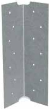
ClarkDietrich EasyClip S-Series™ support clips are commonly used for rigid connections in window and door framing, joist, bypass or other miscellaneous connections to secure one framing member to another, or to secure framing members to the structural frame. This high-performance multi-use utility clip is ideal for corner reinforcements, stair openings and numerous support applications. EasyClip S-Series clips are prepunched for faster and more accurate fastener placement.
