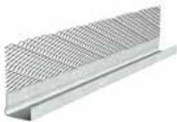
ClarkDietrich veneer trims are J-shaped to fit standard gypsum panel depths with grounds to accommodate veneer finishes. They provide clean, neat edge protection for one- or two-coat veneer plaster finishes at gypsum panel terminations to wall openings and wall or ceiling intersections. Trim with 3/32" grounds is for two-coat veneers and trim with 1/16" grounds is for one-coat veneer plaster.
