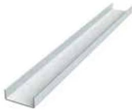
Combined with the deep-leg track clip assembly and EasyClip™ clip angles (U-Series™) or SwiftClip™ (LS-Series), the U-channel creates a traditional assembly that allows for the deflection of floor beams or floor decks above interior partitions. The single, long leg track assembly requires 1-1/2" U-channel and 1-1/2" x 1-1/2" 16 gauge EasyClip or SwiftClip clip angles, installed continuously throughout the uppermost punchouts to align the studs vertically within the plane of the wall.
