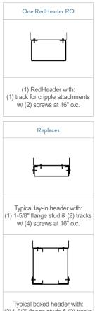
Typical boxed header with: (2) 1-5/8" flange studs & (2) tracks w/ (4) screws at 16" o.c.
