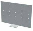
The H-Series<sup>™</sup> universal header hanger is used to connect box headers to jambs, or beams to columns, and transfer large vertical loads. This universal hanger is designed so one part can be used for either side of the connection. The hanger also features a support tab for proper alignment and easy installation.
