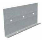
J-weep high-back plaster stop is a J-shaped square-nosed trim manufactured from 26 gauge galvanized steel. Punched weep holes allow for use as a sill weep screed or screed and trim around wall openings. Squared bends accommodate 1" rigid insulation and 3/8" one-coat stucco applications.
