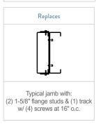
As part of the RedHeader RO system, the jamb eliminates capped members, allowing drywall screws to drive through only one thickness of material. Plus, the open jamb does not require pre-insulating. RedHeader RO Extra-Duty jambs have a longer 3-1/2" flange for wider spans.
