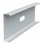
ClarkDietrich C-joist components provide an economical, lightweight alternative to open web trusses, bar joists, engineered lumber, cast-in-place or hollow core floor assemblies. Plus, they're pre-cut to save time. Depending on loads and spans, C-joists are typically spaced at 12," 16," 19.2" or 24" o.c. Joist-togirder attachments are normally supported with joist hangers, EasyClip E-Series™ or S-Series™ support clips. Web stiffeners may be required at supports and other point loads.
