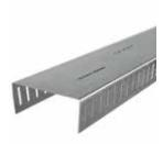
MaxTrak 2D is a head-of-wall deflection track that is used for framing exterior curtain walls and nonload-bearing interior walls where vertical deflection and horizontal drift occurs—and serves as a connecting member that isolates the cold-formed steel framing system from the movement of the primary structure.
