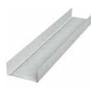
ClarkDietrich C-runner (or H-track) is used to secure H-stud and gypsum shaftliner panels in area separation wall assemblies. Attached to the foundation with powder-actuated fasteners, C-runner is also used as top track to cap the H-stud and gypsum shaftliner panels, with a second track screwed back-to-back to the lower runner, to hold the next assembly level.
