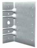
ClarkDietrich EasyClip T-Series™ tall anchor clips are highperformance, cost-effective solutions for knee wall-tofoundation connections, lightduty shearwall-to-foundation connections and truss-to-wall connections. They are designed to resist horizontal, torsional and vertical (uplift) loads.
