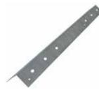
Clinch-On corner bead is recognized as the premier product for providing sturdy metal reinforcement on 90° drywall corners. Knurled and perforated flanges offer superior compound adhesion for smooth, straight finishes. Corner bead attachments are accomplished by nailing, stapling, screwing or clinching through the flanges.
