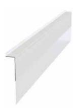
Platinum reveal trims are used to finish wallboard terminations when the board abuts other building materials—such as suspended ceilings, beams and untrimmed door and window jambs—to create a clean step inset or reveal. Helps create aesthetic architectural detailing around light fixtures, ceilings, walls and soffits, without mechanical fasteners.
