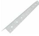
Clinch-On hot-dipped corner bead offers the identical roll-formed precision as its counterpart. Hotdipped galvanized metal corner bead (meets ASTM C1047) provides enhanced corrosion protection and sturdy reinforcement at exposed 90° corners. Flanges are knurled and perforated to ease joint compound adhesion and nail attachment.
