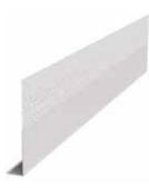
Platinum L-trims are used to finish the ends of wallboard where it abuts dissimilar surfaces, such as suspended ceilings, beams, plaster, masonry or untrimmed door and window jambs. Applied in the same manner as all other tape-on beads joint compound embeds the paperfaced bead to the wallboard paper.
