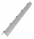
The TradeReady<sup>®</sup> Spazzer<sup>®</sup> 9200 bar is a pre-notched, 20 gauge, galvanized steel spacer and bridging bar. It facilitates rapid erection of studs into a rigid, accurately laid out gridwork that has excellent resistance to stud rotation and displacement. Hanging drywall is also faster and easier because the Spazzer 9200 bar eliminates the bow that often occurs in tall interior studs.
