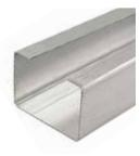
Headers are prepunched, and pre-cut to the length specified on your order. Header depth is 1/8" narrower than jamb depth to accommodate fit into HDSC Clip. Header lengths should be ordered 1/2" shorter to fit inside clips.
