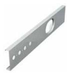
ClarkDietrich TradeReady® steel joists clear spans up to 33 feet, and are one of the primary components of the TradeReady floor system. Large extruded holes accommodate HVAC, mechanical, plumbing, electrical and sprinkler runs. The joist also features a series of smaller holes for electrical and technology lines. Hole sizes range from 4-1/4" oval to 10" round, based on member depth.
