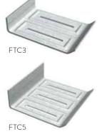
ClarkDietrich Fast Top<sup>™</sup> clips are used in head-of-wall deflection conditions for in-fill curtain wall assemblies to provide for vertical movement. These clips are used in place of, or in combination with, deflection track. They also make a positive attachment and eliminate the need to install bridging continuously throughout the uppermost punchouts. Attach to the underside of structural members, concrete decks or floor assemblies.
