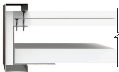
Jamb trim grouted in place and/or attached to J-Tabbed Track with jamb anchor clips
