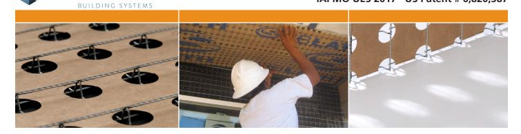
V-Truss Walls & Ceilings (Structa Rib Lath) is designed for superior performance of stucco on overhead surfaces. V-Truss Walls & Ceilings is a self-furring welded wire lath for use as an alternative to 3/8" 3.4/yd<sup>2</sup> rib metal lath specified in ASTM C 847 for use in Three-coat stucco and as an alternative to the 1.4 lb/yd<sup>2</sup> woven wire lath specified in ASTM C 1032.
