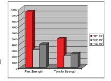
**Tensile Strength:** This number describes how large of a load a panel can withstand before it breaks due to elongation. Higher numbers indicate materials that can withstand a stronger pull before breaking. *(Test Method ASTM D638/D651)*
