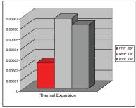
**Thermal Expansion:** This is a measurement of how much the length of a material will change when the material is heated or cooled. The graph shows how much the material will increase in length if the temperature of the material is raised one degree Fahrenheit. Smaller numbers indicated relative stability to changes in temperature. (**Test Method ASTM D256**)
