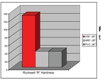
**Rockwell "R" Hardness:** Measures a material's surface hardness. A steel point is forced into the material and its resistance to penetration is measured. *(Test Method ASTM D785)*
