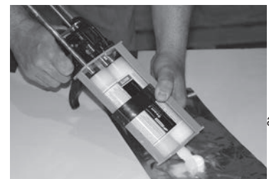
FIGURE 13: LEVELING THE PLUNGERS
