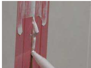
Figure 19: Bump adhesive in to previous section
