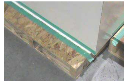
Figure 22: Horizontal seam filled completely with sealant
