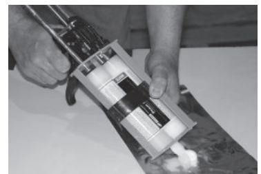
FIGURE 13: LEVELING THE PLUNGERS
