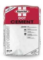
**CURING:** Most materials made with Rapid Set® DOT CEMENT must be water cured. Keep exposed surfaces wet for a minimum of 1 hour. Begin curing as soon as the surface starts to lose its moist sheen. When experiencing extended setting time due to cold temperature or the use of retarder, longer curing times may be required. The objective of water curing shall be to maintain a continuously wet surface until the product has achieved sufficient strength.
