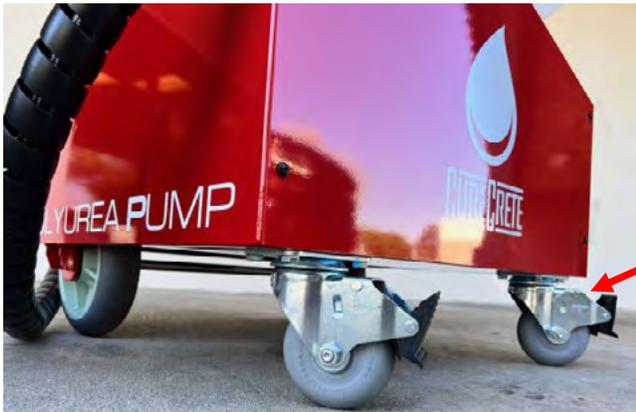
Heavy duty rounded swivel casters with brakes
