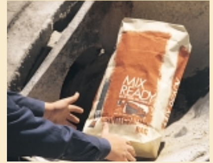
11. Disintegrating bags of color additives can be tossed into a mixer without opening or pouring.
