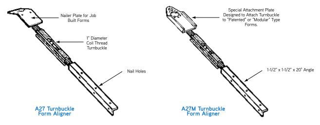
Dayton Superior A27 and A27M Turnbuckle Form Aligners are designed to accurately position and plumb vertical forms. The turnbuckle section of the aligner features a 1" diameter self-cleaning coil thread for fast adjustments. Overall length of the aligner is 37" minimum and 40" maximum, offering 3" of effective adjustment.
